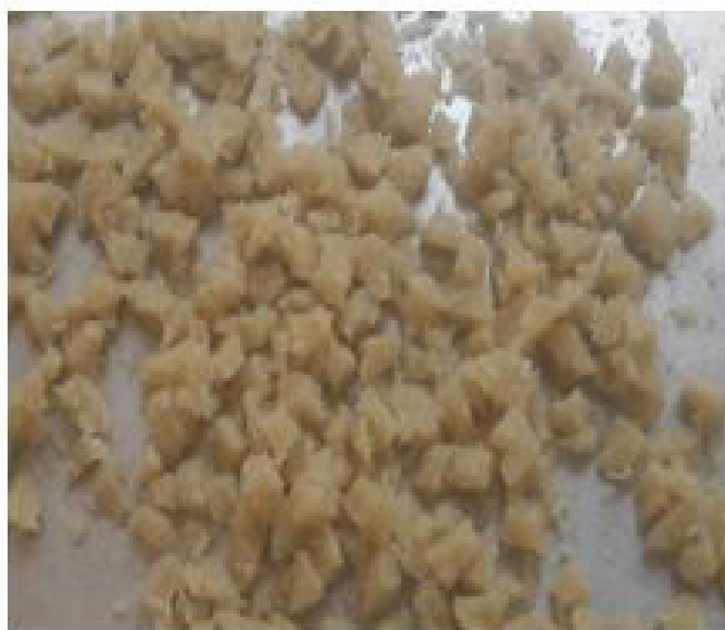
Figure 1: Dried hydrogels utilized as PPG in this study
