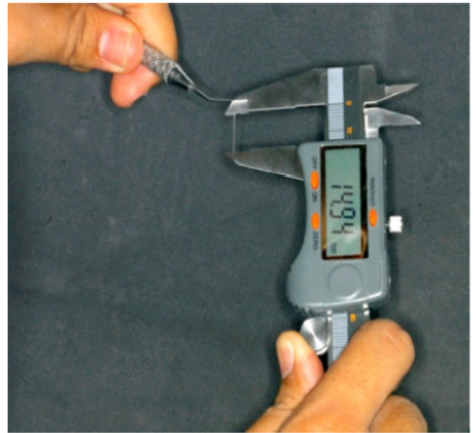
Figure 2 - Measurement of a PCP-15 type probe in the 0.015.0 mm marking parameter, according to the adopted methodology.
