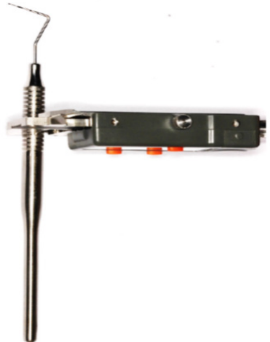
Figure 3 - WHO periodontal probe perpendicular to the ground under cable diameter analysis (lateral view).
