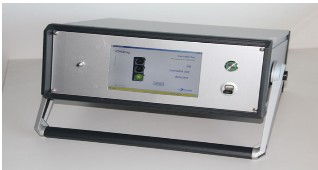
Figure 5 The mobile GC-IMS IONdrug with ~ 8 kg incl. a battery for 4 h autonomous operation.
