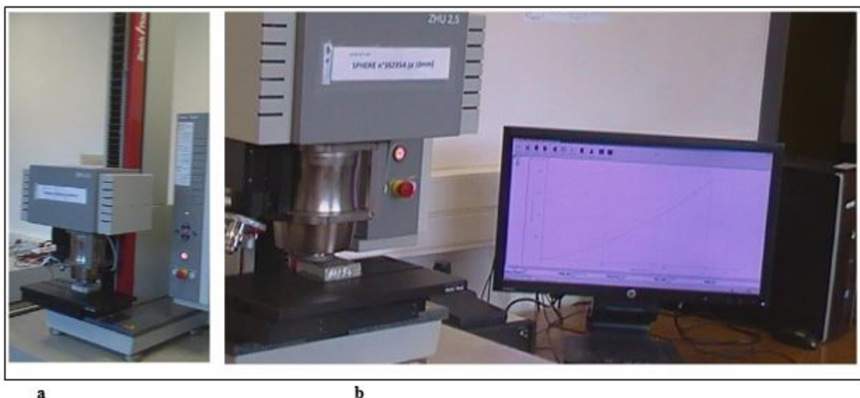
Figure 4: instrumented indentation test set-up: (a) General view of the macro indenter Zwick and (b).zoom on the two cells of observation and indentation
