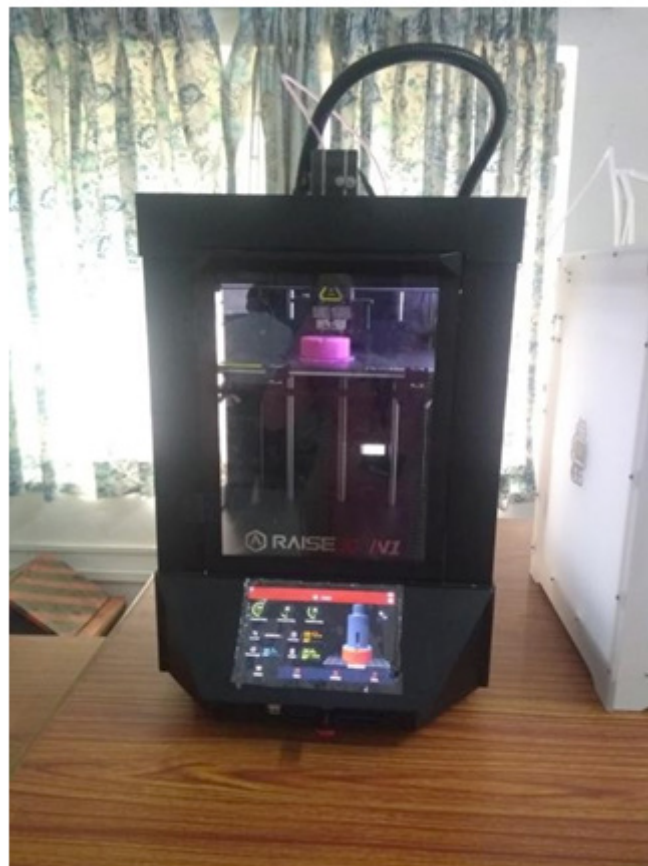
Figure 1: Fused deposition modeling machine (Courtesy: Vasavi College of Engineering)
