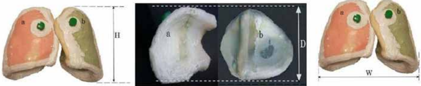
Figure 1: The dimensions of the anatomical lung phantoms a) the right lung b) the left lung. (Height: H = 23 \text{ cm} , Width: W = 28 \text{ cm} and Depth: D = 13.7 \text{ cm} )
